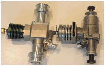
play when the drive shaft is rocked in it, but is good when running. A slot is easier, but the Oliver style carb direction would be better to use here as there would not be much metal "meat" left if the slot was in the
