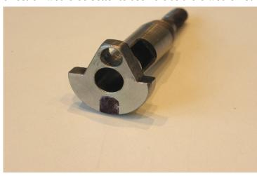
crankpin position, because of the counterbalancing cut outs in the Enya crankweb, as can be seen. I have marked the position and shape for a slot in black here, 180 degrees opposed to the hole. Now, Peter recommended rebalancing the Enya shaft by removing metal from the crankweb as needed, which is a bit of a specialist job, though I skipped this and my engine runs well without it.
