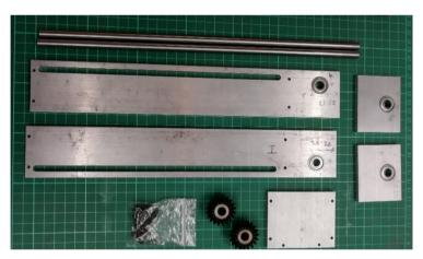
the gear hubs do not rub on the race outers. The actual size ended up at 62.26mm giving an overall width of 74.96mm because the side panels are ¼" (that's why you have DROs on machines...) The gears were from Amazon – look for 'Mxfans 2 x Modulus 1.5 Silver 8mm Hole 20T Tapered Bevel Gear Wheel with Top Screws' or similar.
